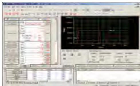
Profile Trace (On-line) Monitoring operation speed of each axis with graph type and saving result as image file.
