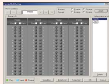
Forced I/O The status of external output device can be checked without program. And when input device breaks down, forced input function specifies ON/OFF and can operate the system without interruption of equipment.
