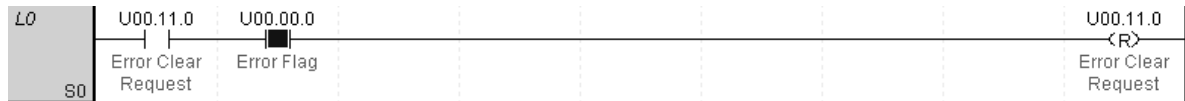
[How to use the flag to request error clear ("S" type or "H" type)]
