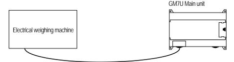
For No Protocol Communication, one of following end condition is designated. One is the size of the received data, and the other is the the received data setting that is the some with pre-defined data.
