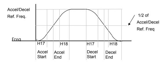
▶ Note that setting Frequency Ref. for Accel/decel (H70) is set to Max Freq and target freq is set below Max freq. the shape of S-curve may be distorted.
