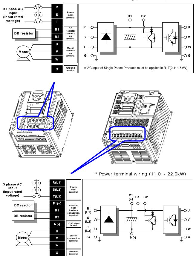
2.4 Specifications for power terminal block wiring
