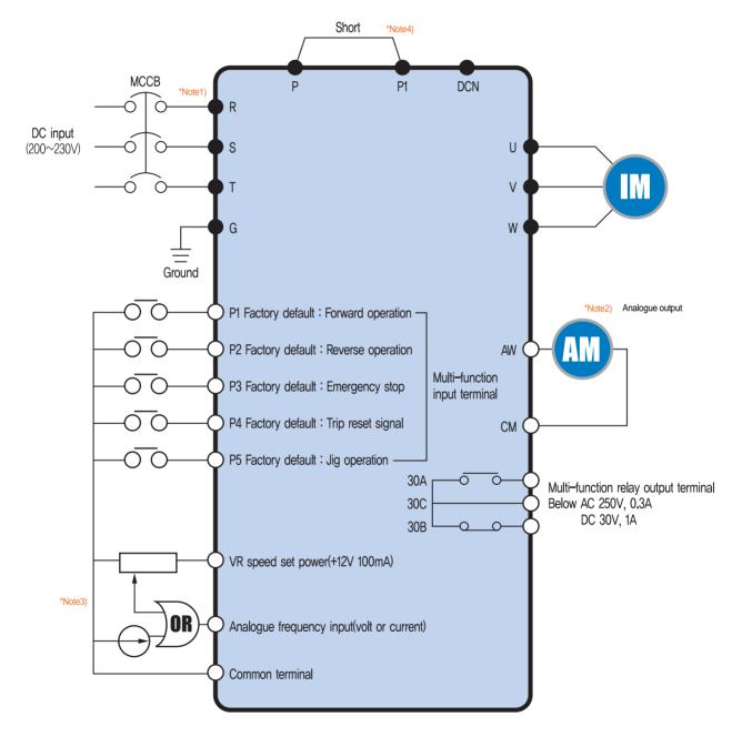
\*Note1)" 'and" 'means the main circuit and the control circuit respectably.
