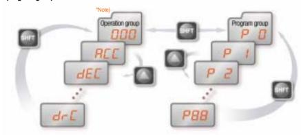
\*Note) The target frequency can be set at the first group of operation group so that the factory default value has been set as 0.0 yet in case of frequency change, the changed frequency is displayed.
